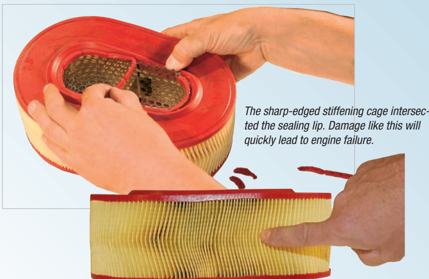
Strongly deformed filter medium causes a tearing of the filter paper.
