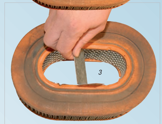
The sharp-edged stiffening cage intersected the sealing lip. Damage like this will quickly lead to engine failure.
