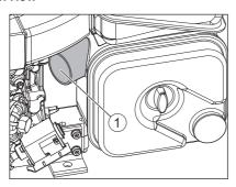
1 Intake opening for combustion air
