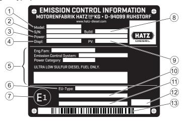
The engine type plate is affixed to the crankcase and includes the following engine information:
